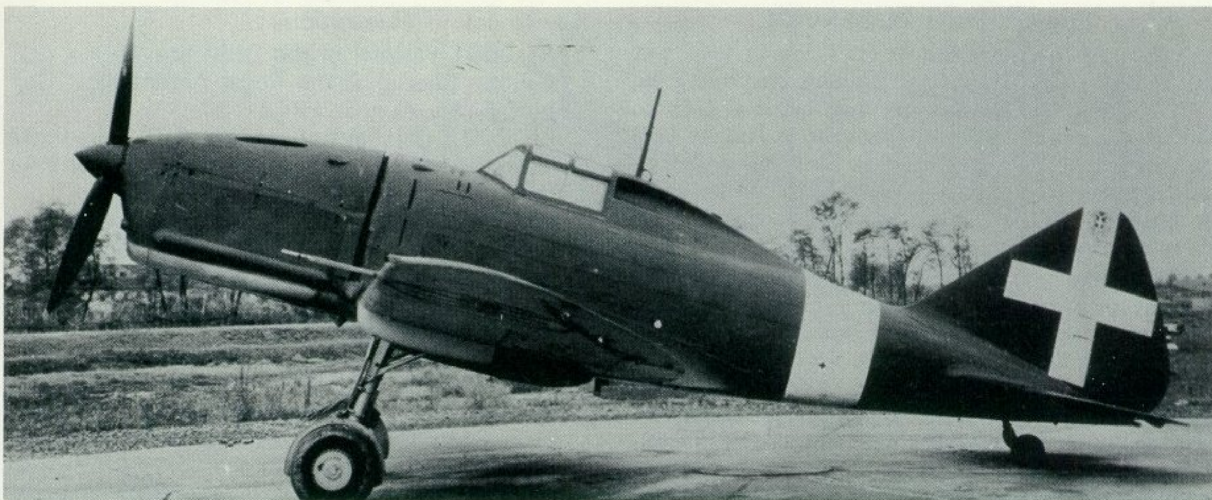
The sole example of the Re 2001 Delta (serial MM9920). This aircraft was lost in an accident on January 27, 1943. Apart from its powerplant and the altered nose contours, the Re 2001 Delta was similar to the standard version.
