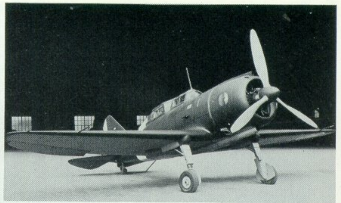
The first prototype Caproni Reggiane Re 2003 two-seat reconnaissance aircraft (serial MM478). Only two Re 2003s were built.
