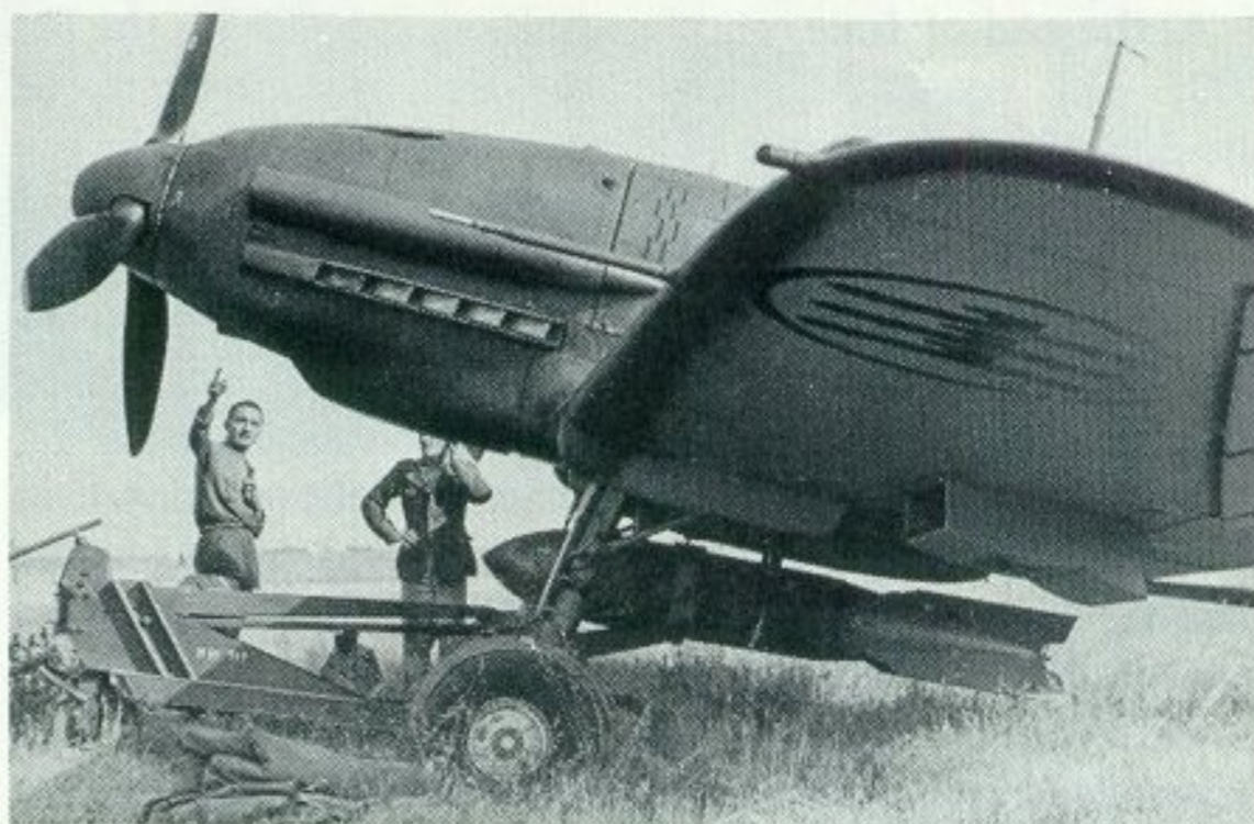
The sole example of the Re 2001 Delta (serial MM9920). This aircraft was lost in an accident on January 27, 1943. Apart from its powerplant and the altered nose contours, the Re 2001 Delta was similar to the standard version.
