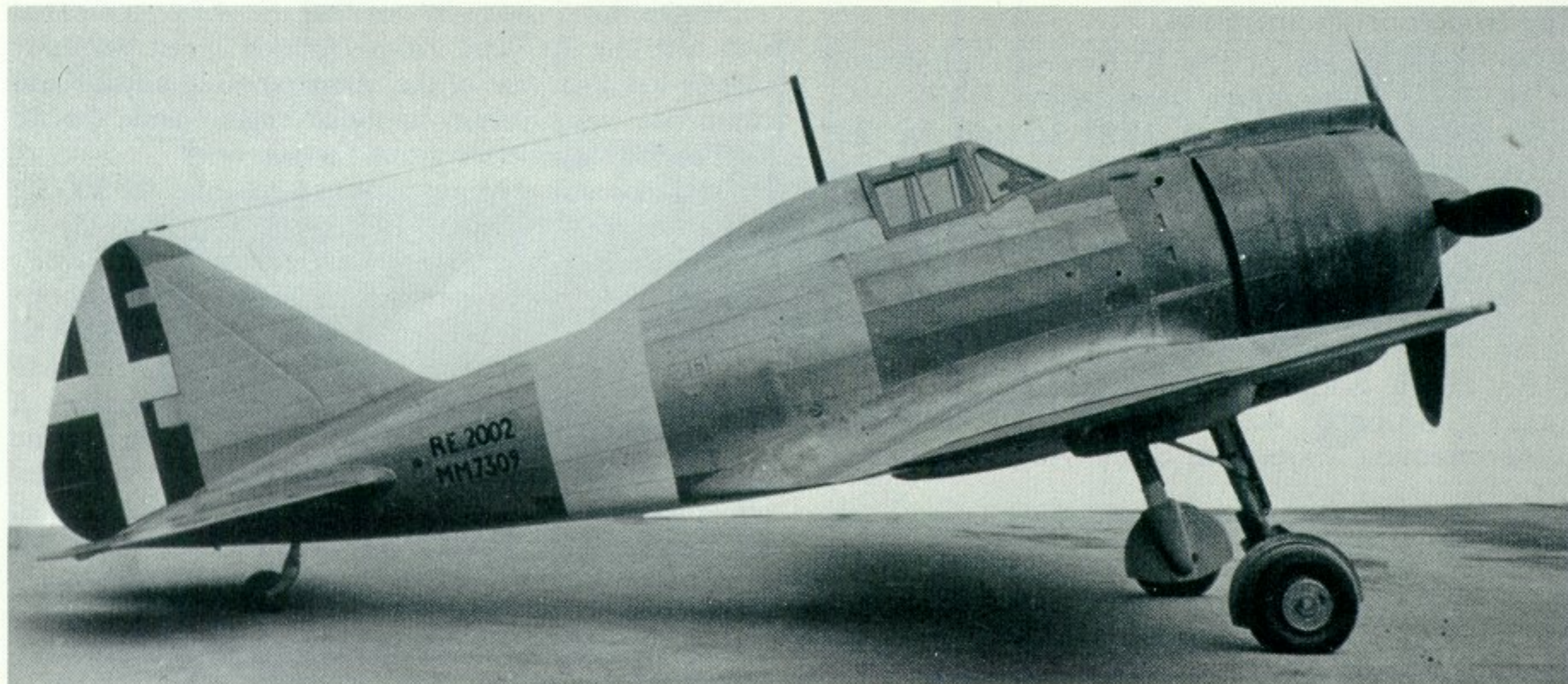
The production prototype Re 2002 (serial MM7309) had a redesigned engine cowling and spinner, modified cockpit canopy and fixed tailwheel. (Photo: Museo Aeronautico Caproni di Taliedo)
